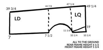
The maximum combined length of door and quarter together, front to back, is as follows:
